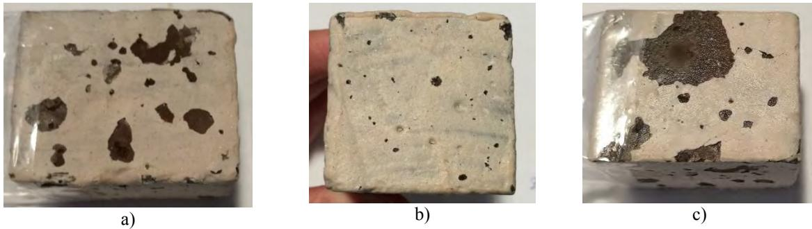
**FIGURE 5.** Visual appearance of the cube sample 23 coated with zircon paint after 1500 hours in contact with the molten salts in surface A, B and C.
