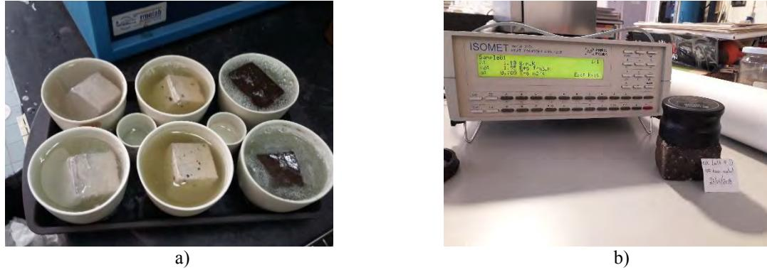
**FIGURE 1.** a) Bath of concrete samples and molten salts references in crucibles. b) Thermal measurement after 1000 hours of contact with molten salts.
