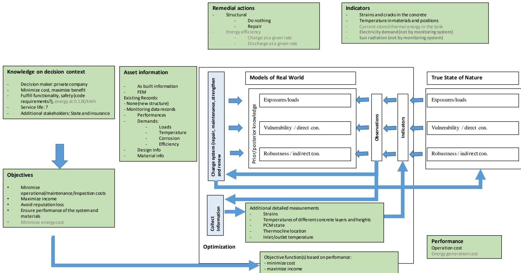
Figure 6: FlowChart for SMS concrete thermocline tanks.
