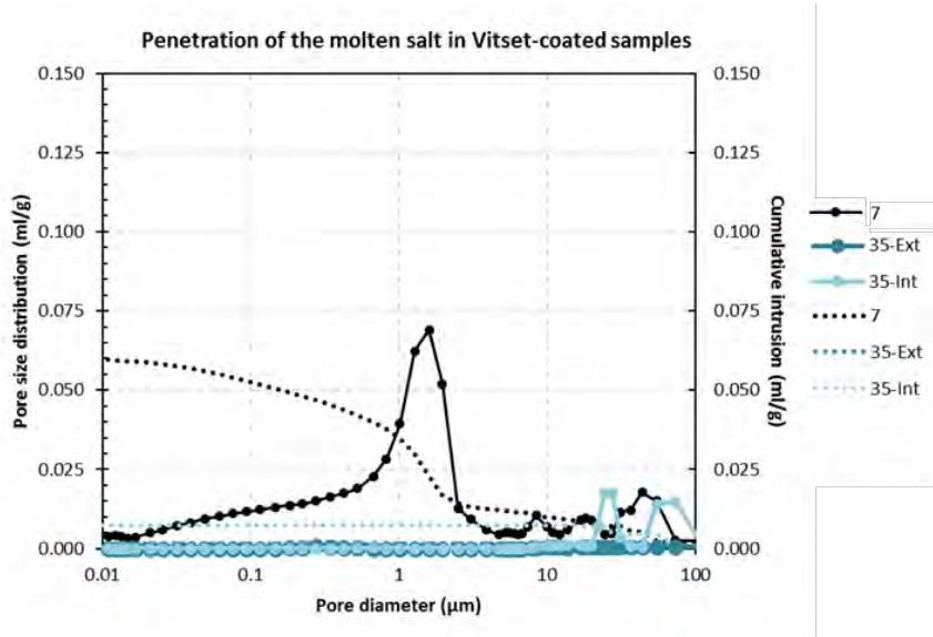
**FIGURE 10.** Pore size distribution for a reference concrete sample (7) and two zones of a sample coated with vitset mortar after interacting with Ternary mixture under thermal cycles for 1500 hours. (note: solid lines show the pore size distribution curves, principal axis, and dashed lines cumulative intrusion curve, secondary axis)
