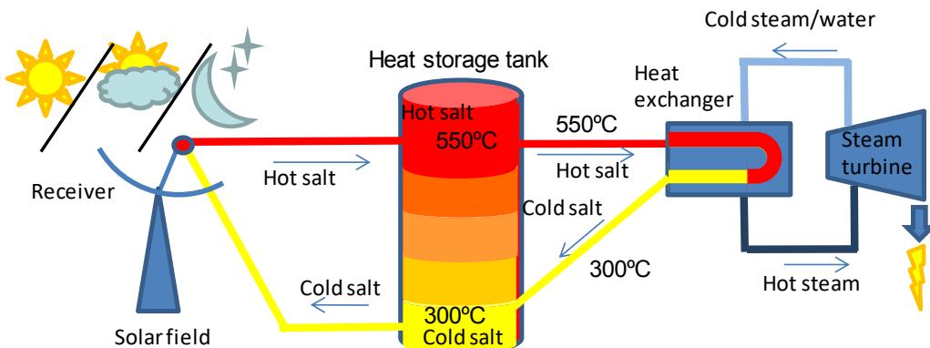
Figure 3: Thermocline SMS tank configuration on a CSP
