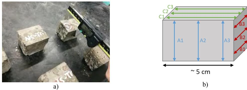
**FIGURE 3.** a) Measure of the thickness of the cubes before the application of the coating. b) Three directions of the measurements performed on the prisms.
