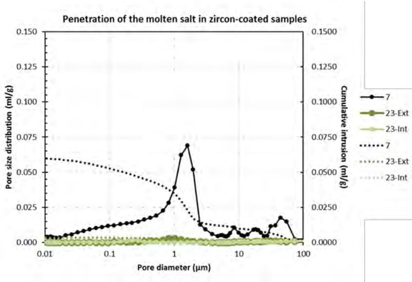
**FIGURE 9.** Pore size distribution for a reference concrete sample (7) and two zones of a sample coated with zircon paint after interacting with Ternary mixture under thermal cycles for 1500 hours. (note: solid lines show the pore size distribution curves, principal axis, and dashed lines cumulative intrusion curve, secondary axis)
