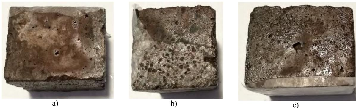
**FIGURE 4.** Visual appearance of an uncoated cube after 1500 hours in contact with the molten salts in surface A, B and C.
