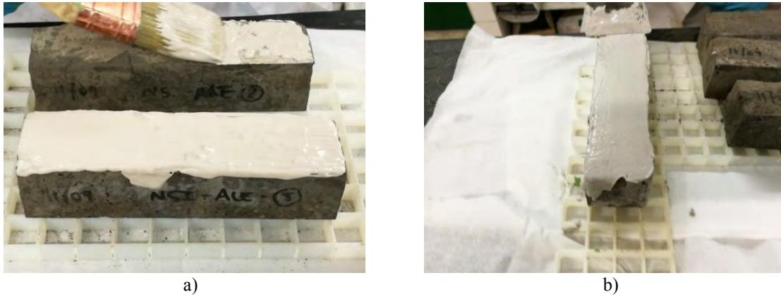
**FIGURE 2.** a) Application of the paint with a brush. b) Application of the mortar with a spatula.
