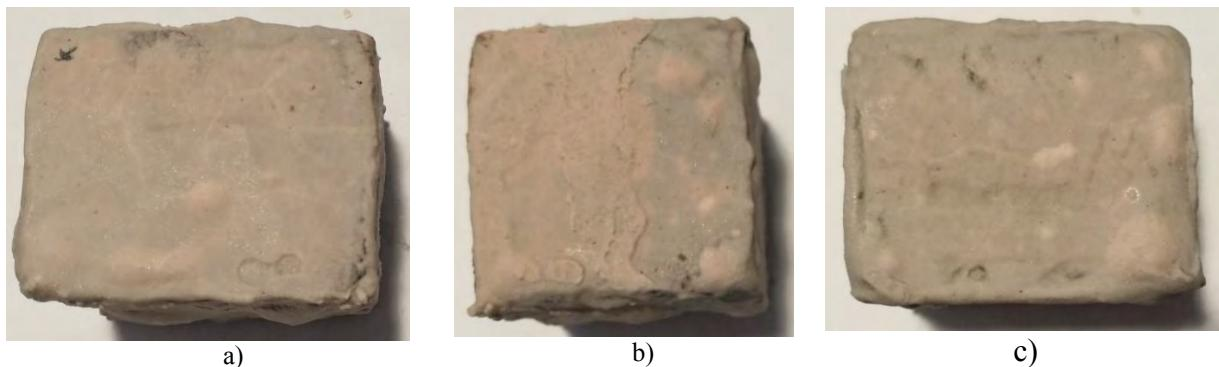
**FIGURE 6.** Visual appearance of the cube sample 35 coated with vitset mortar after 1500 hours in contact with the molten salts in surface A, B and C.
