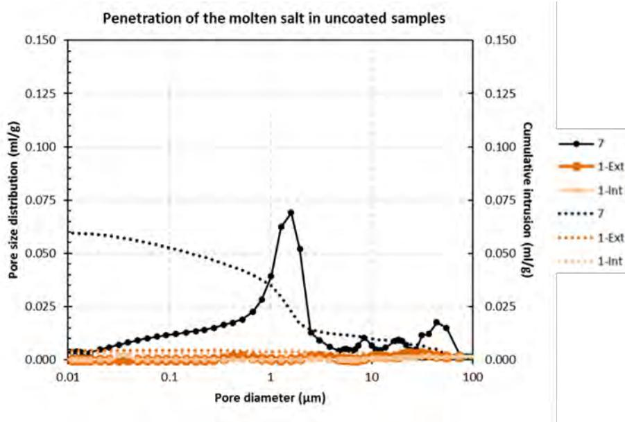
**FIGURE 8.** Pore size distribution for a reference concrete sample (7) and two zones of a sample after suffering the contact with ternary mixture after 1500 hours. (note: solid lines show the pore size distribution curves, principal axis, and dashed lines cumulative intrusion curve, secondary axis)
